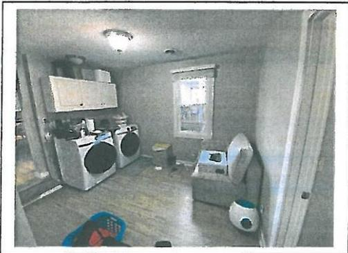
**Scope:** To build a new bathroom in the area where the laundry is now. Demo the existing wall and floor finishes to expose the frame cavities. Frame the new walls for the bathroom divider wall and laundry separation wall.
